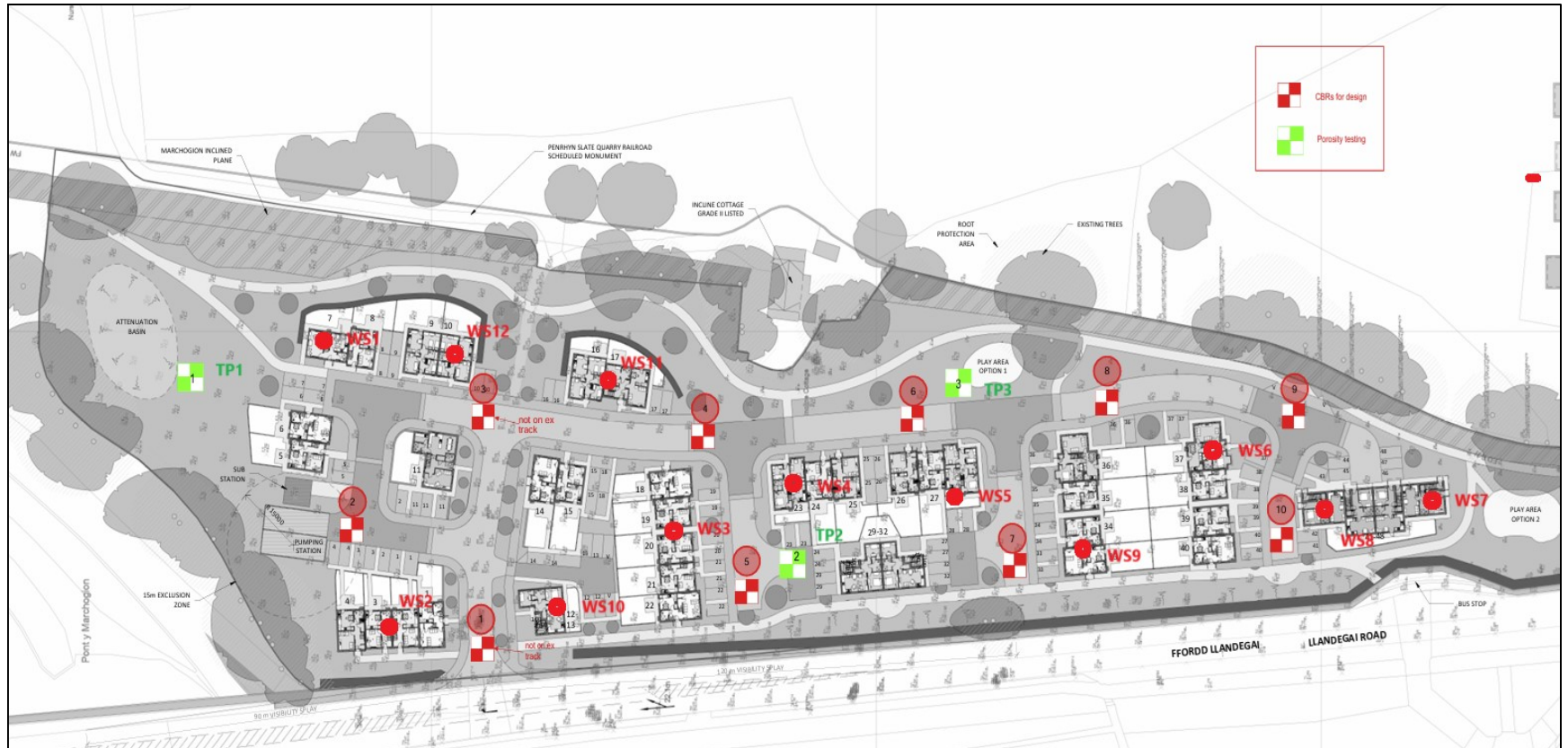
Figure 4 – Window Sample Boreholes (WS1 to WS12), Trial Pit Locations (TP1 to TP3), CBR Locations (CBR1 to CBR10)
