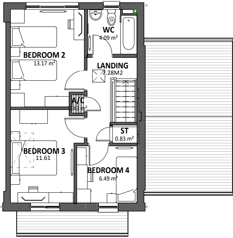
FIRST FLOOR PLAN SCALE: 1 : 100
